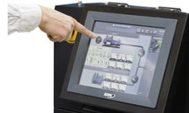
The new APM802 command/control system is specifically designed for operating and monitoring power plants for markets including hospitals, data centres, banks, the oil and gas sector, industries, IPP, rental and mining.
